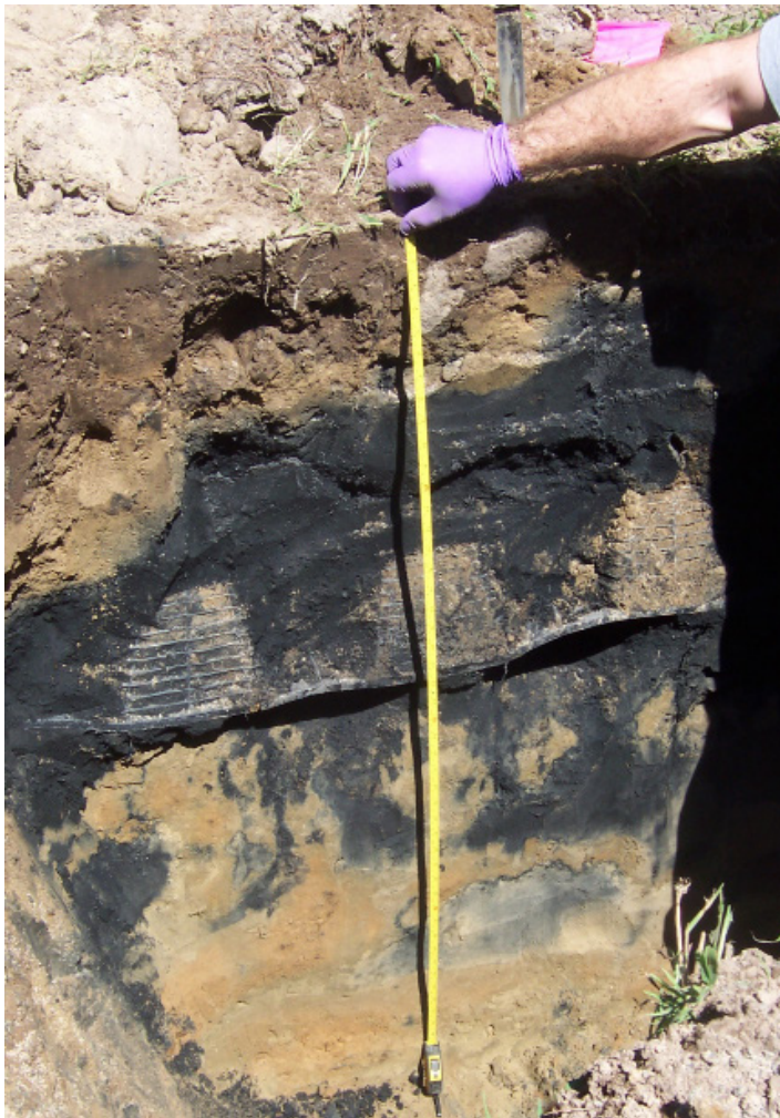
Organic staining (black color) below, along-side and above a failed soil absorption field trench. Vents of plastic chamber are visible.
